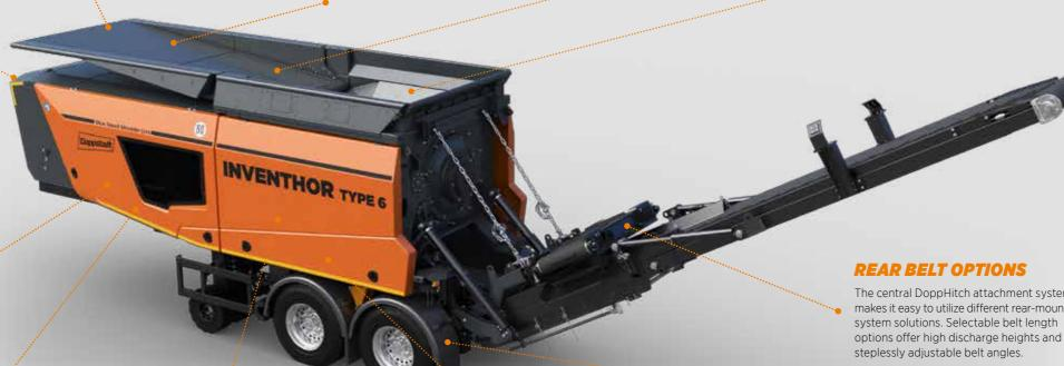
The central DoppHitch attachment system makes it easy to utilize different rear-mounted
